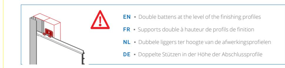
**EN** • Double battens at the level of the finishing profiles
